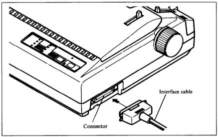
Figure 1-6. Connecting the interface cable
