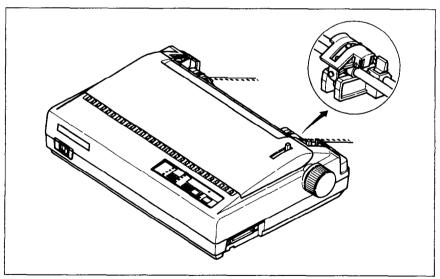
Figure 1-11. Closing the sprocket covers
