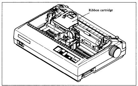
Figure 5-1. Replacing the ribbon cartridge
