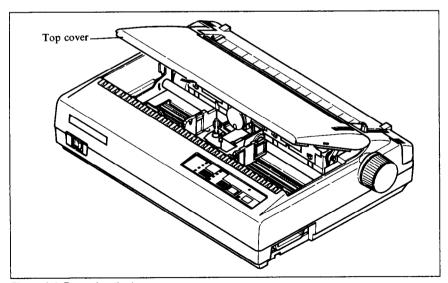
Figure 1-4. Removing the top cover
