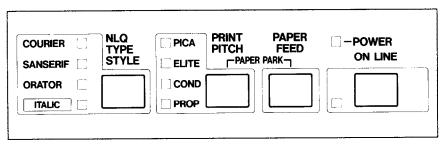
The control panel switches can be pressed singly to perform the operations indicated by their names. Other functions can be obtained by holding these switches down when you turn the printer's power on. Still further functions can be executed by pressing the control panel switches in combination. This chapter explains all the switch and indicator functions.
