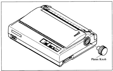
Figure 1-3. Mounting the platen knob
