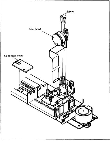
Figure 5-2. Replacing the print head
