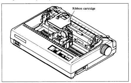
Figure 1-5. Installing the ribbon cartridge
