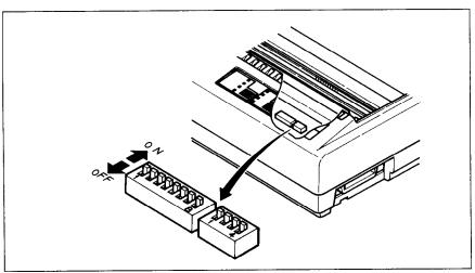
Figure 1-15. DIP switches
