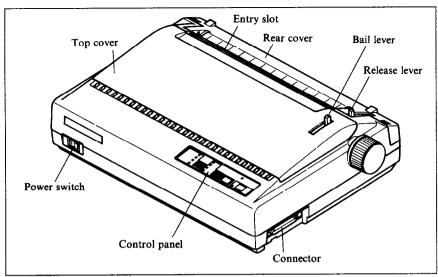
Figure 1-2. The printer's external parts
