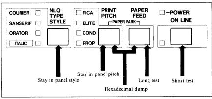
Figure 2-4. Power-up functions of control panel
