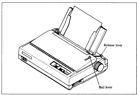
Figure 1-8. Loading a single sheet
